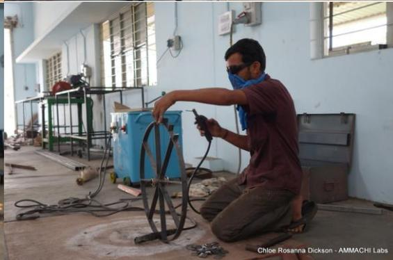
Back and front wheels were made by bending and soldering steel sheets (1" wide for back wheels). Spikes were cut out of a 90° extrusion, opened up and welded to the wheel. The front rim is connected to a standard bicycle wheel hub. The back wheels have a pipe (1" inside) as a hub.
