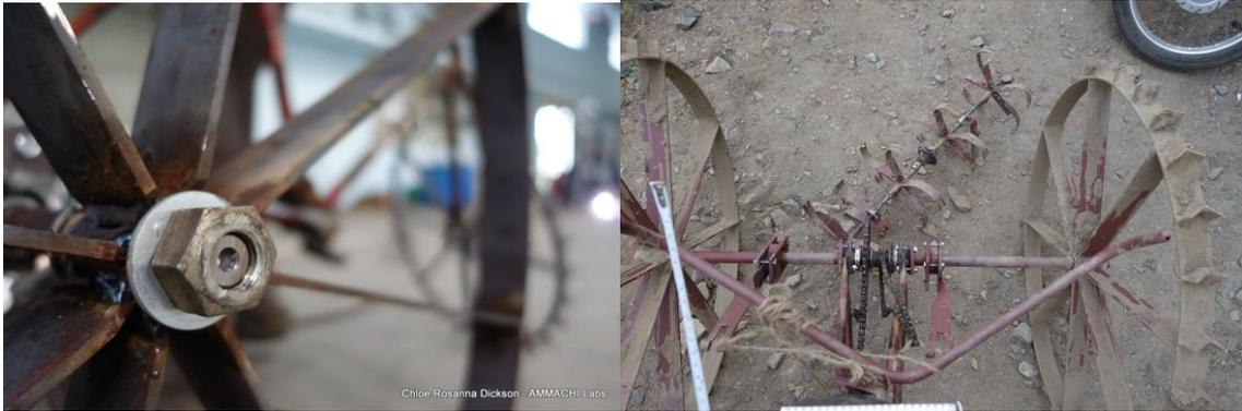
The main axle is a 1" rod with threaded ends. The wheels are resting on the threading and bolted tight. On smooth ground and while driving straight, the wheels are both driving. When taking curves, the inside wheel slips on the axle, enabling sharp turns. This may cause problem on highly uneven ground where both wheels may slip.
