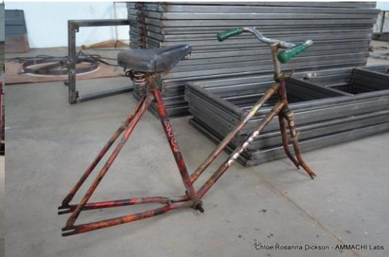
For this prototype, a second hand ladies' bicycle was used. Wheels, gear set, brakes and accessories were removed. Wheel hubs, sprockets and crank set were kept aside.
