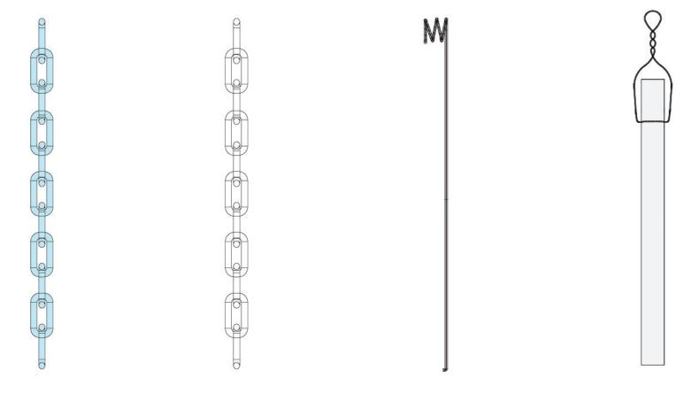
METAL CHAIN: Worked OK on harder beans and rye but not as well PLASTIC CHAIN: Worked well on larger beans that weren't as dry STAINLESS STEEL BICYCLE SPOKES (14G)
