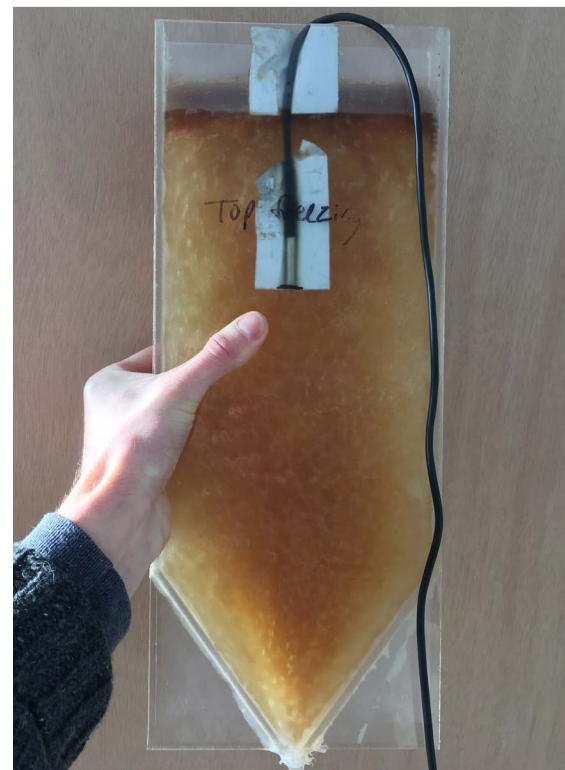
Frozen urine in experimental freeze concentration chamber.
