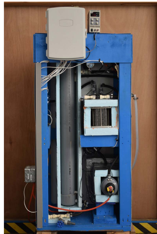
Electric resistance pasteurizer with heat exchanger for energy recovery.
