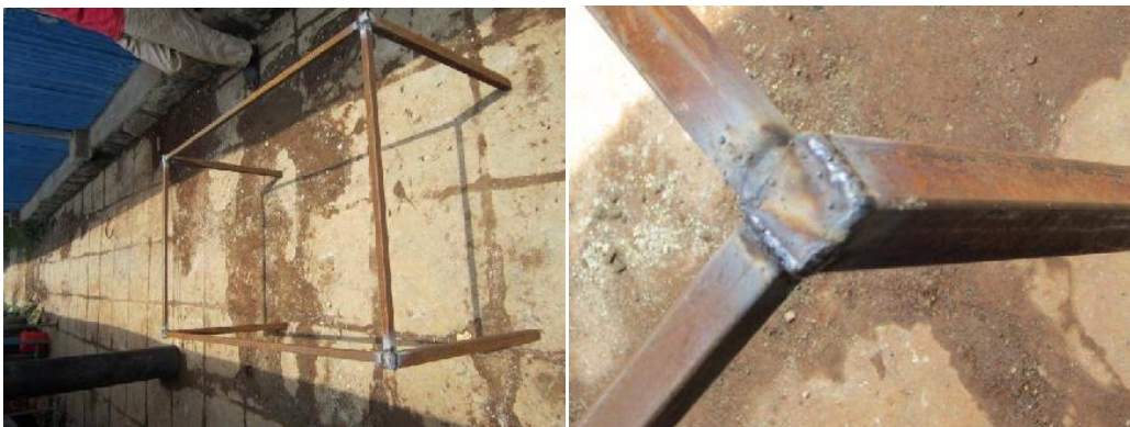
Picture 5: image of feet attached (left) close-up view of feet attached (right)
