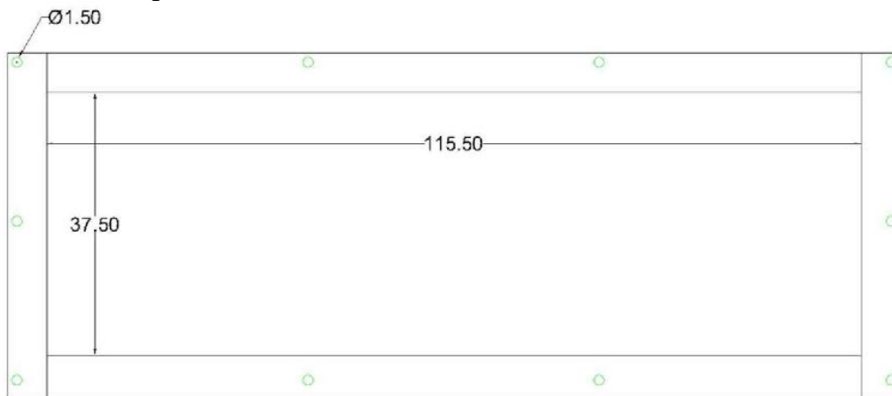
Figure 47: Dimensions for baking chamber flange bolt holes
