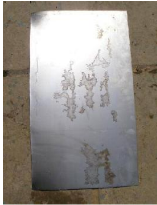
Picture 9: Back plate of combustion chamber
