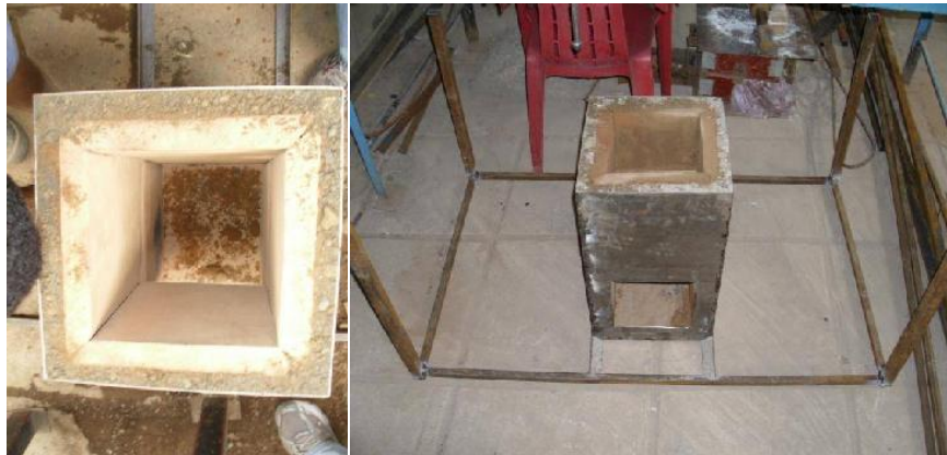
Figure 23: Addition of last tile (left) and complete combustion chamber (right)
