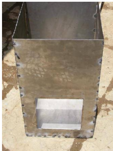
Picture 10: Completed metal combustion chamber
