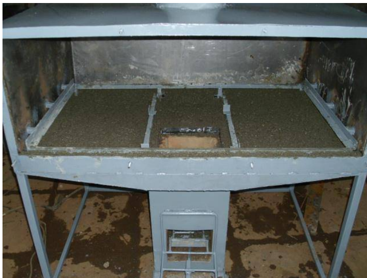
Picture 85: Pumice/concrete layer added to the taper
