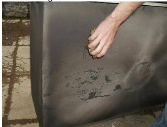
Picture 91: Image of cleaning outer surface of baking chamber
