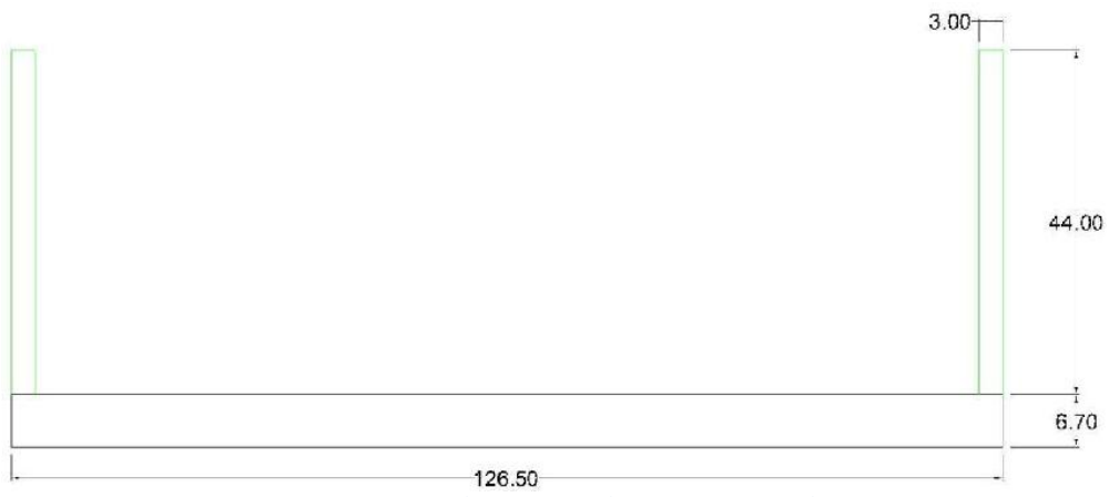
Figure 40: Dimensions for the sides of the oven chamber flange
