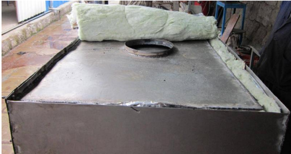
Picture 64: Image of top fiberglass piece added
