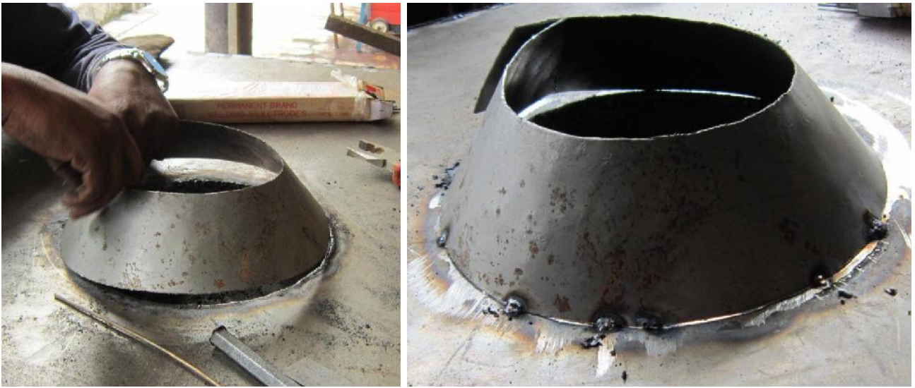
Picture 67: Images of manifold shaped to fit hole (left) photo of manifold spot welded on with excess material (right)
