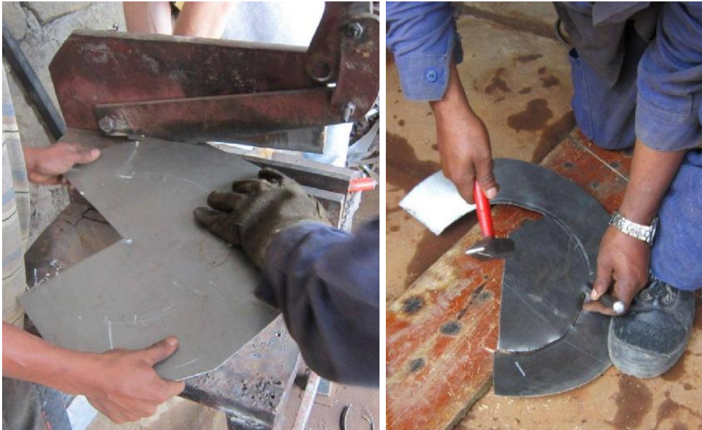
Picture 66: Images of manifold being cut
