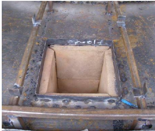
Picture 55: Image of angle bar placeholders for baffle
