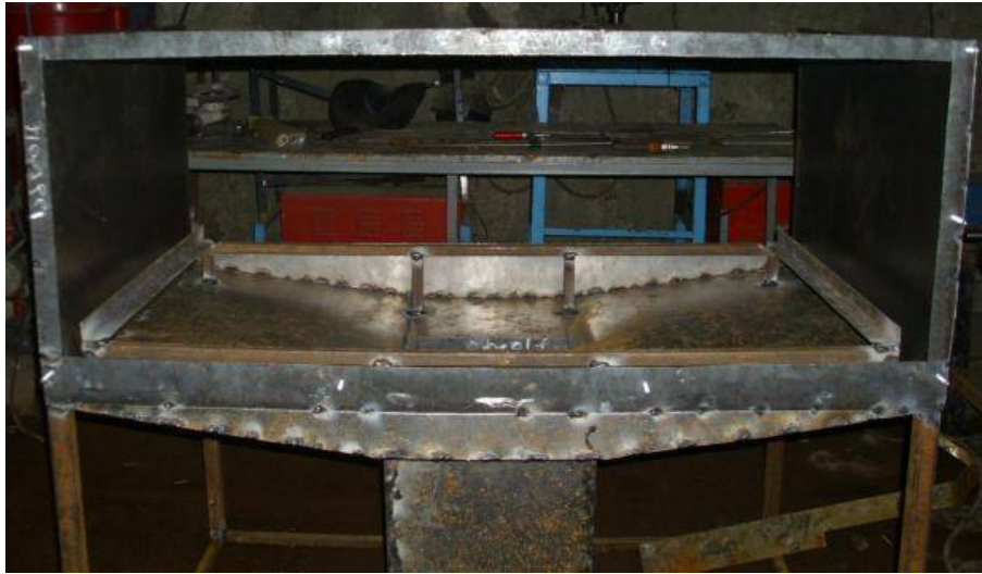
Picture 53: Image of oven chamber lip attached
