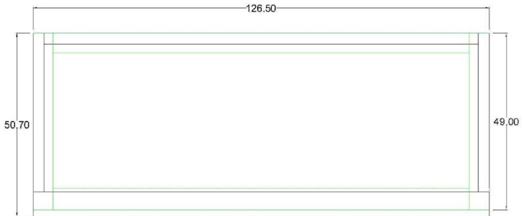
Figure 44: Oven chamber flange (black) on top of baking chamber flange (green)
