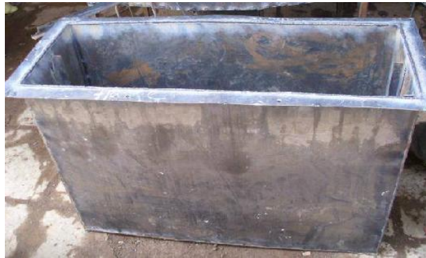
Picture 36: Flange welded onto the baking chamber
