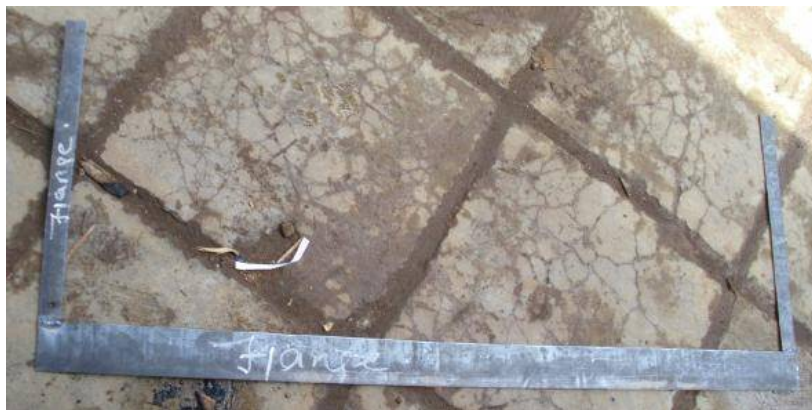
Picture 26: image of the sides of the oven chamber flange attached
