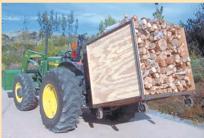
Simple firewood-hauling box attaches to the 3-pt. hitch on Ron Ziegler’s Deere 5205 tractor. It rolls around easily on caster wheels at the house.
