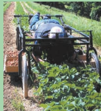
“I built it almost entirely out of old bicycle parts,” says Francis Voegeli about his berry-picking cart that’s “paddled” by the operator.
