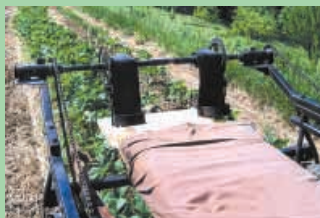
The operator lays down on the cart to pick (right) and moves himself down the row with a pair of foot paddles (above) that drive bicycle sprockets and chains through a nifty ratchet system.
