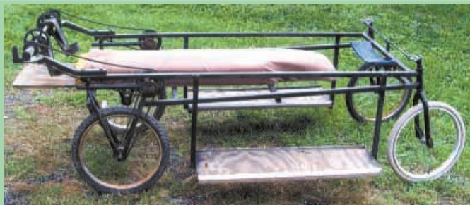
“I built it almost entirely out of old bicycle parts,” says Francis Voegeli about his berry-picking cart that’s “paddled” by the operator.
