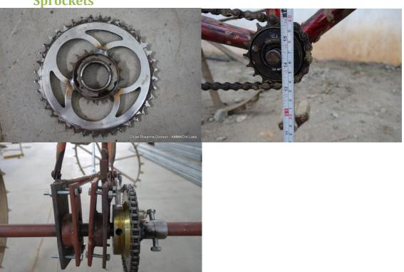
Front and back sprockets were reversed for easy pedalling as high speed is not required for envisioned agricultural applications. The front chain ring was welded on a back sprocket and freewheel attached to the back axle. The back sprocket was welded in the front to the crank set. A test was also made with a 10/50 gear set bought on the market which further reduced the speed and required operation force. The alignment (both vertical and horizontal) caused friction and derailing issues.
