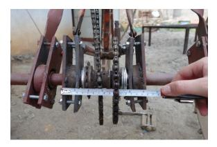
The bicycle frame is connected to the back wheels axle by 1" bearings welded to the frame with an intermediate piece allowing easier removal. One part of the bearing "sandwich" contained the bearing itself and was attached to the axle. The opposite part of the sandwich was shaped as an open "C", welded to the bicycle frame and to be fitted around the bearing and bolted in place.
