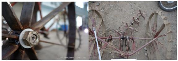
The main axle is a 1" rod with threaded ends. The wheels are resting on the threading and bolted tight. On smooth ground and while driving straight, the wheels are both driving. When taking curves, the inside wheel slips on the axle, enabling sharp turns. This may cause problem on highly uneven ground where both wheels may slip.
