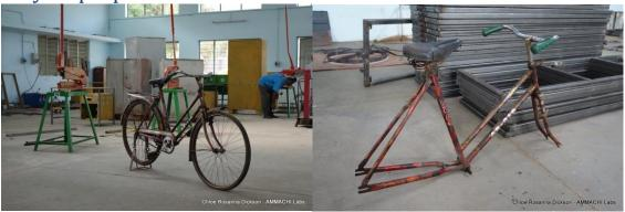
For this prototype, a second hand ladies' bicycle was used. Wheels, gear set, brakes and accessories were removed. Wheel hubs, sprockets and crank set were kept aside.
