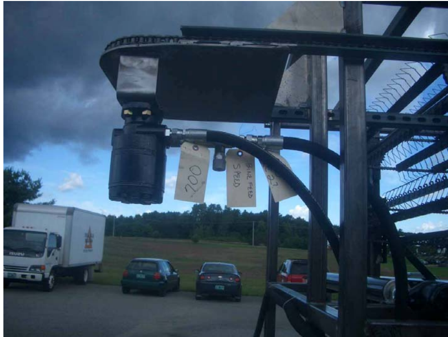
Figure 7. Bine feed motor, mount, and speed control valve on the front (feed inlet) side of the machine).
