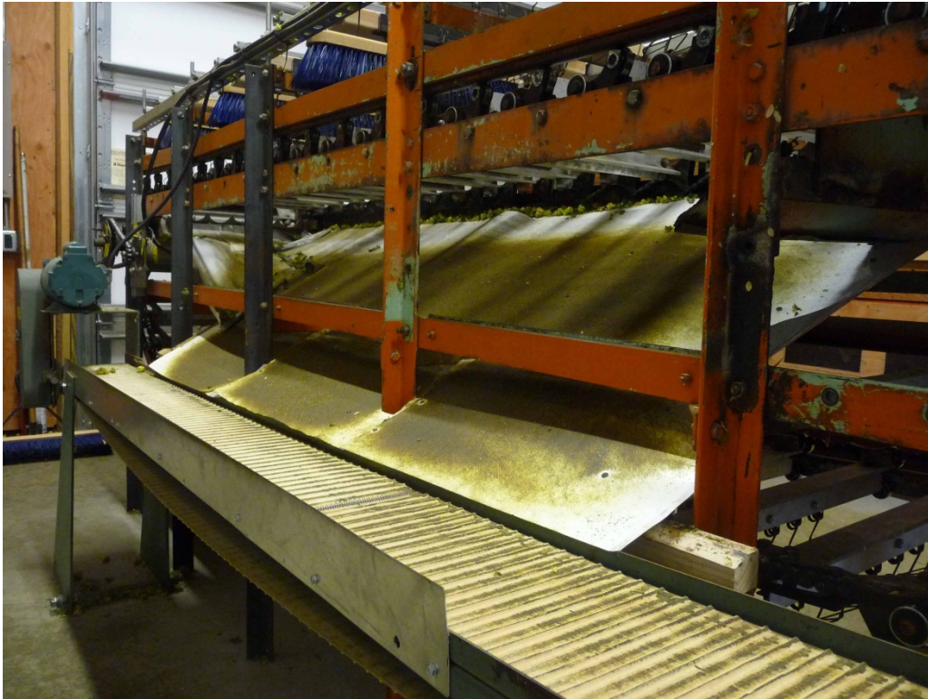
Figure 9 - Cone collection chute and conveyor. (Photo credit: Rich Andrews)
