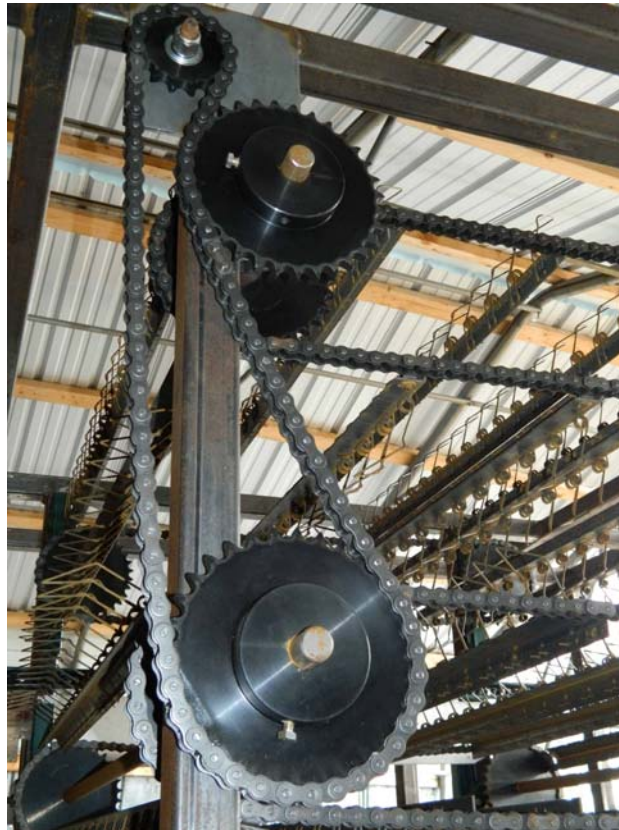
Figure 13. Reversing transmission is required to make the top stripping belt run in the same direction as the bottom.
