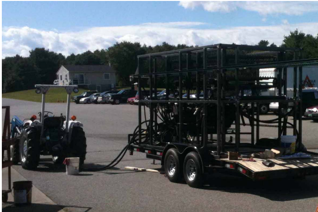
Figure 24. The harvester with the PTO pump connected on a small tractor for initial testing.
