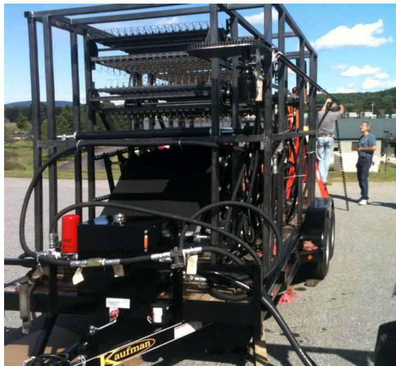
Figure 6. Harvester on the trailer with only stripping section and dribble belts installed. Bine feed extension is being assembled on far end of picture.
