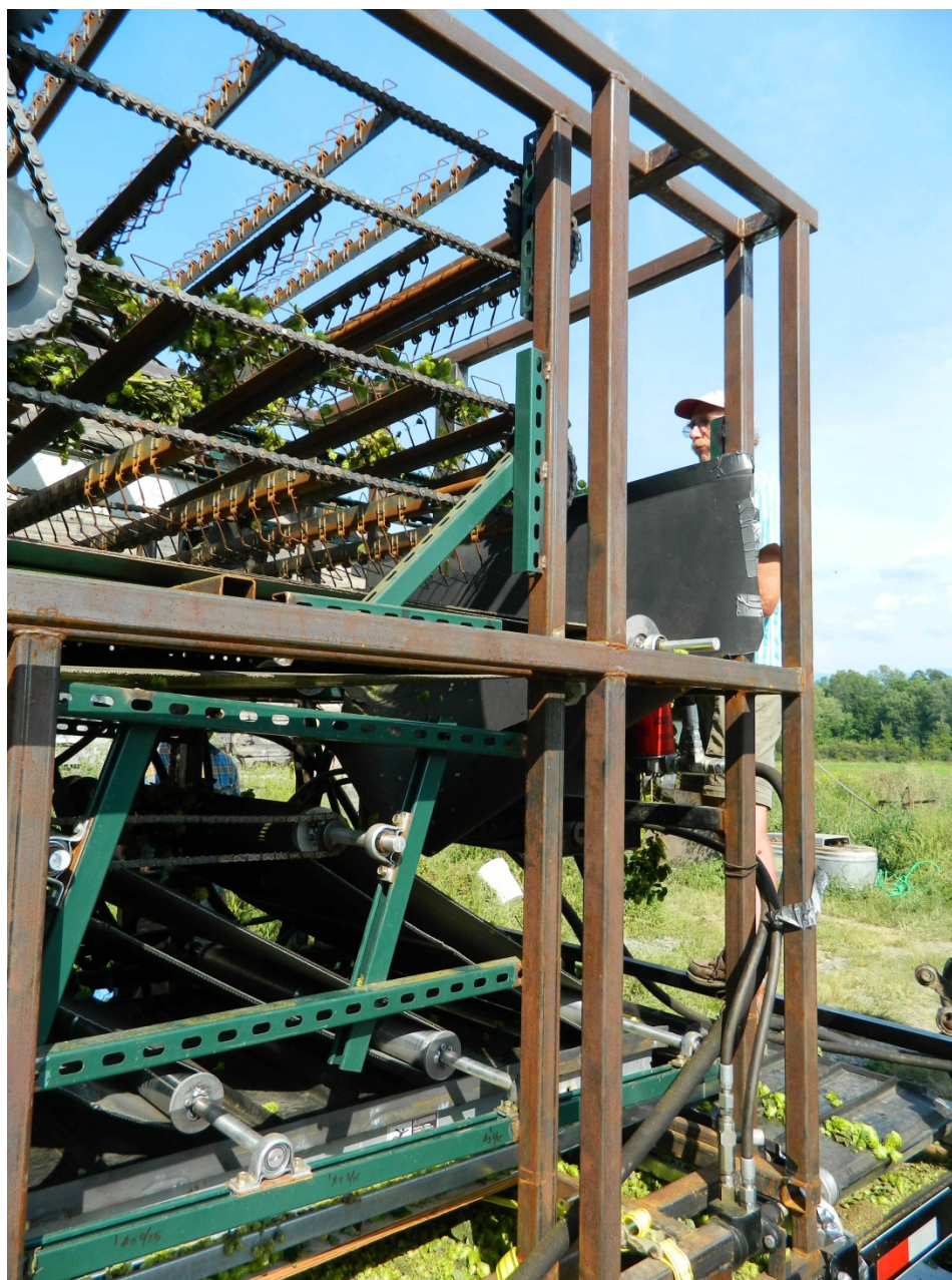
Figure 4 - The trial inlet chute that directs stripped cones to the dribble belts is visible in this view (black PVC sheet).
