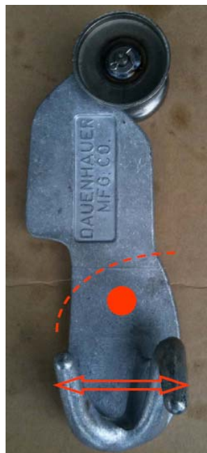
Figure 4. A bine hook purchased from Dauenhauer Manufacturing Co., Inc. Due to space limitations in the bine feed area of the stripping section we had to trim the hook as shown by the dashed line. We also drilled a new hole for attachment to the bine feed chain using attachment links. Lastly, we had to reverse the bine hook finger locations since we were pulling the bines down the right side of the machine.
