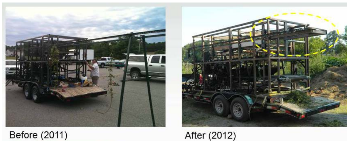
Figure 1 - The bine feed was shortened on the exit end and was also moved to be centered in the stripping section.
