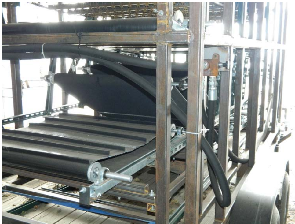
Figure 20. Trash conveyor viewed from back end of the machine. When operating it brings leaves and twigs from the last dribble belt out the back of the machine. As noted above, the belt does not need to be cleated.
