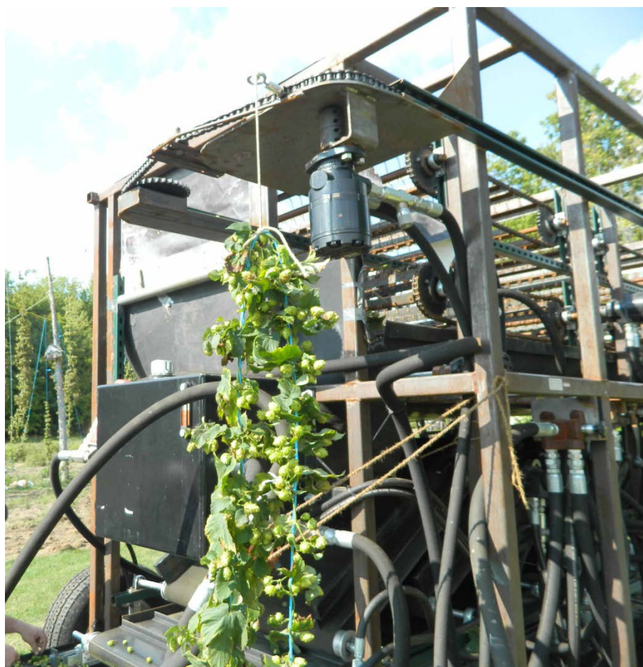
Figure 2 - The new location of the bine feed is now centered. The cord used for bine attachment is also shown in this view.
