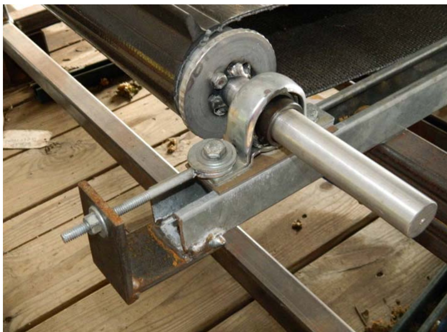
Figure 21. All long conveyors (strippage, primary hop, secondary hop, and trash conveyors) required a tensioning adjustment. This was accomplished in the prototype using a long eye bolt fastened to the corresponding pillow block bearing using the existing bolt and UniStrut lock nut.
