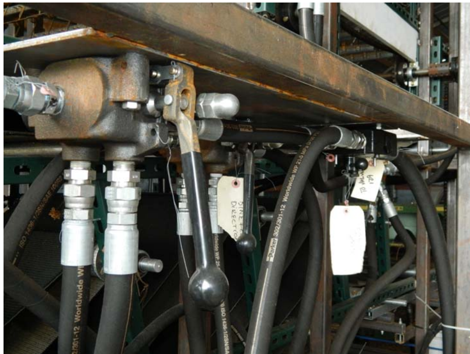
Figure 28. Three control valves. The nearest is the bine feed directional control valve (a three position, single spool control valve, Valve #303). A second of the same type is the next valve to the right and is used to control the stripper section direction (Valve #203). On the far right side of the picture is the stripper speed control valve mounted upside down (Valve #129). See Bill of Materials and Hydraulic Schematic for more information.
