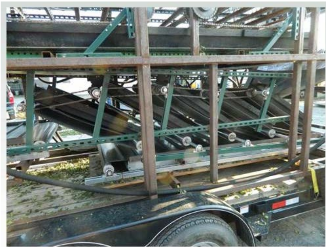
Figure 3 - Containment fences are be seen on the primary conveyor and dribble belts in this view.
