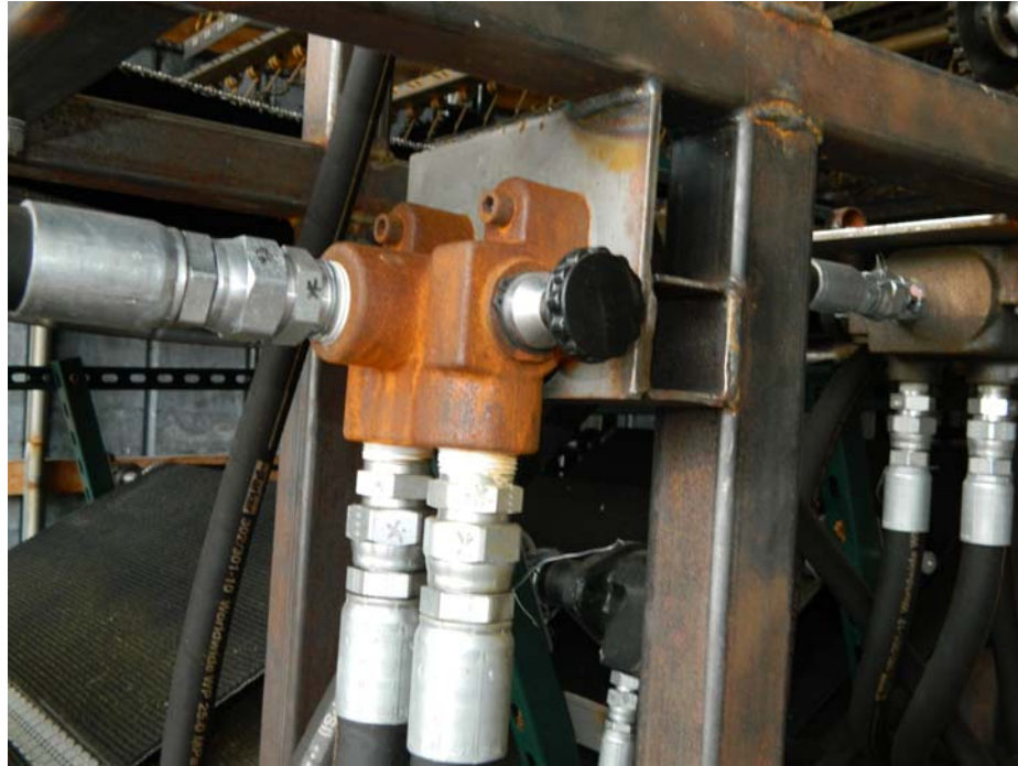
Figure 27. A single spool two position valve used as an emergency stop switch for the machine (Valve #'s 117 & 123). Two are included on the machine at opposite corners. When pushed in, they shunt all hydraulic flow directly from the pump to the reservoir, depowering the motors. Either of the two valves will do this. The valve spool needs to be pulled out in order to run the motors again.
