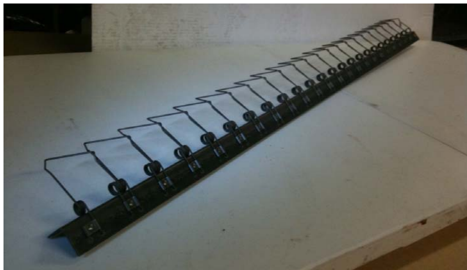
Figure 11. Stripping fingers mounted on a 48" bar, purchased as an assembly from Dauenhauer Manufacturing Co., Inc. The fingers / bars are attached to the stripping chains so that the tip of the finger leans slightly away from the incoming bine (i.e. away from the direction of stripping finger travel.)
