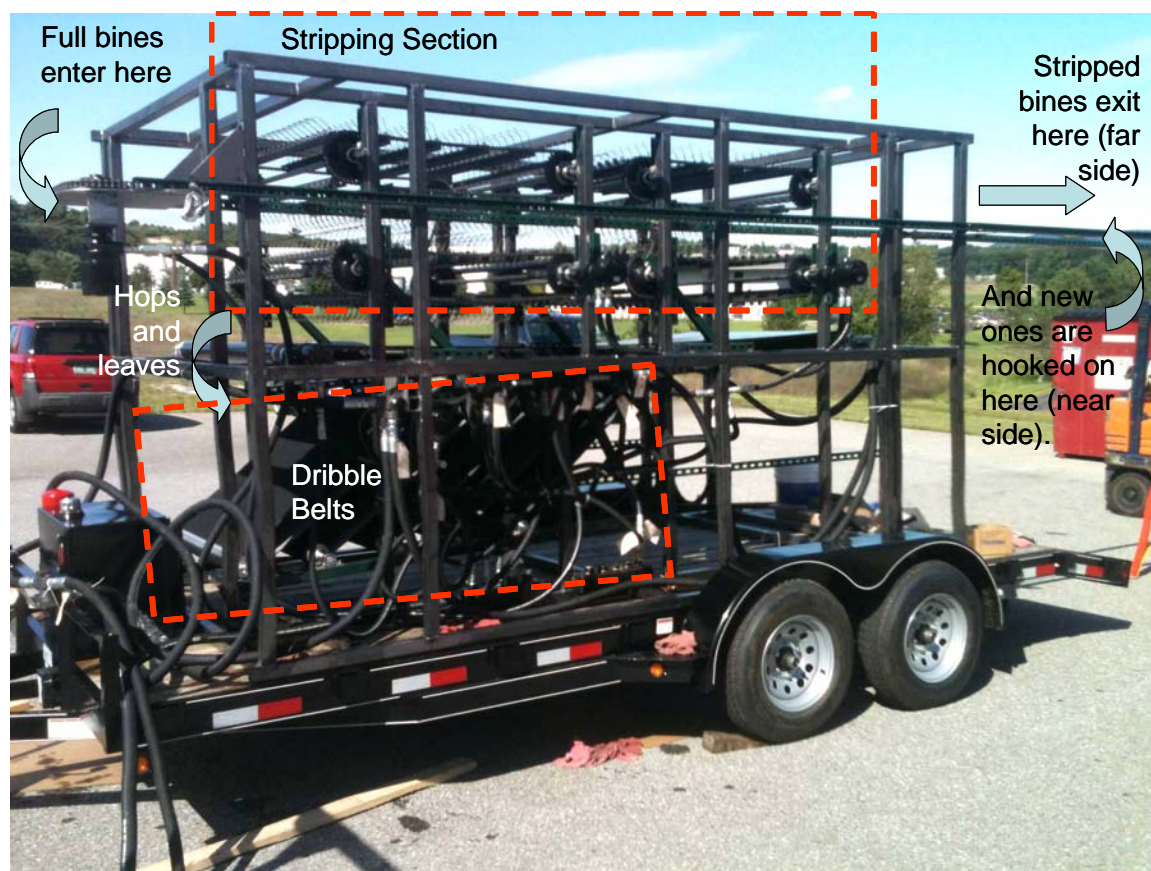
Figure 1. Photo of the harvester during initial test, showing main sections in place.
