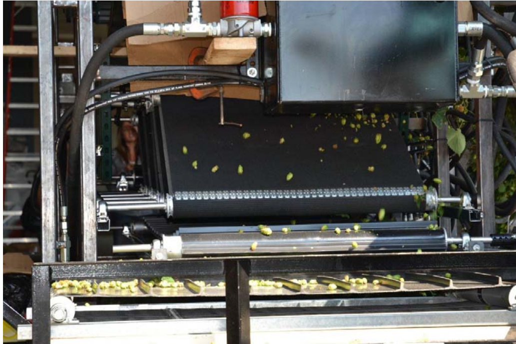
Figure 19. The dribble belts at work, viewed from the bine feed inlet (front) side of the machine. The cardboard in the photo was used to direct all strippage onto the dribble belts as panels and chutes had not yet been fabricated for that purpose. Primary and secondary hop conveyors are also visible in this photo, with “sorted” cones being delivered to the left of the photo.
