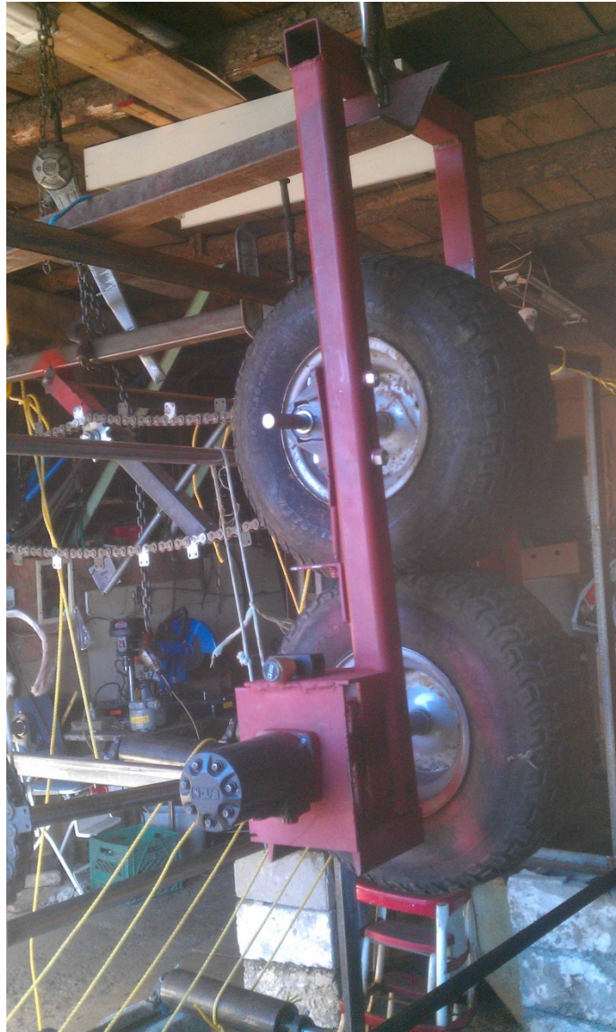
Figure 12 - Daniel chose two lawn mower tires to pinch and pull the bine through the stripping section. (Photo credit: Daniel Sabourin)
