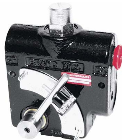
Figure 26. Flow control valve used to set stripping assembly speed by controlling the split of flow between the stripper motors and all other motors. (Valve #129)
