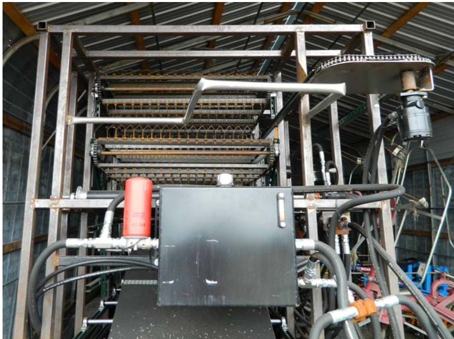
Figure 5. The bine feed inlet (front) of the machine. Showing the bine feed motor, chain, sprockets and mounting plate in the upper right corner of the picture.
