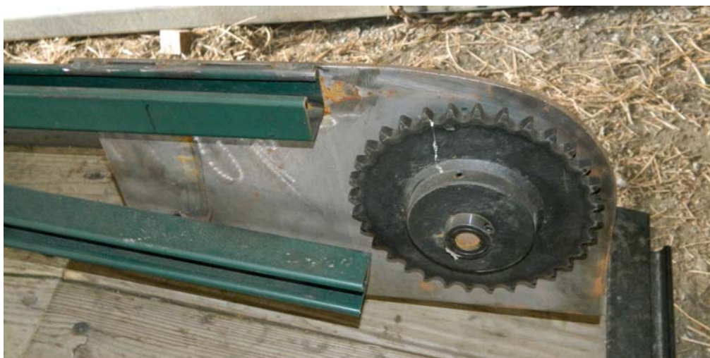
Figure 8. The far end of one half of the bine feed extension showing idling sprocket and mounting plate. Chain not attached in this photo.
