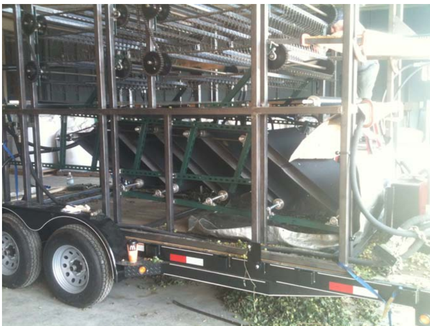
Figure 15. A side view of the machine showing the relation of the dribble belts to the stripping belts and how the dribble belt drive chain is connected between belts.
